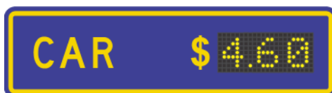
Figure 4.6(b) – Electronic panel for toll road price information
