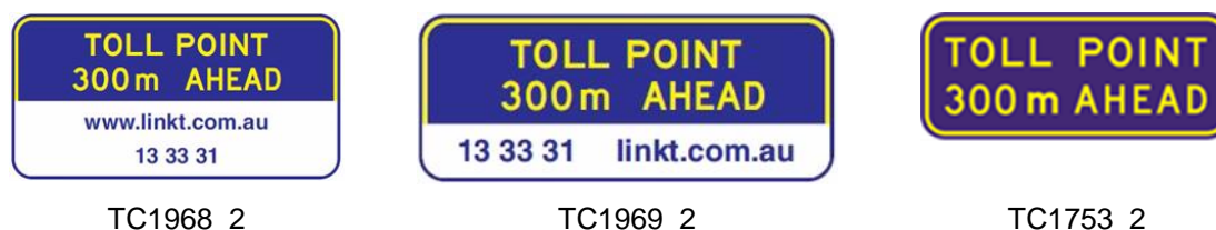
Figure 4.1(b) – Extra signs used in advance of toll point
