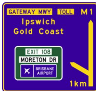
Figure 7.2(c) – An exit to a toll road from a non-tolled road
