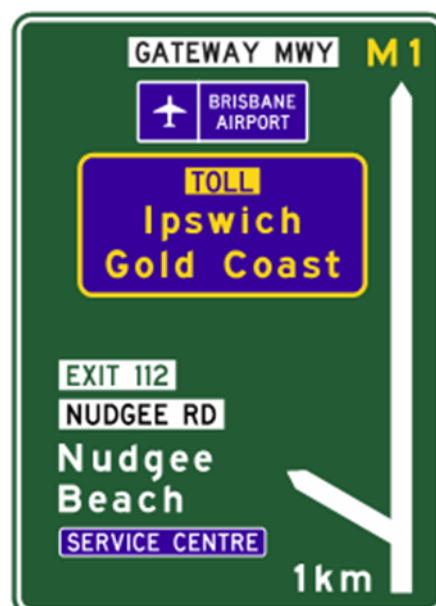
Figure 7.1(c) – Example, Toll road patch and colour scheme, not on immediate approach
