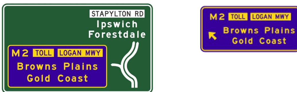
Figure 7.14 – Direction signs for an ENTRY to a toll road with a toll point on the on ramp
