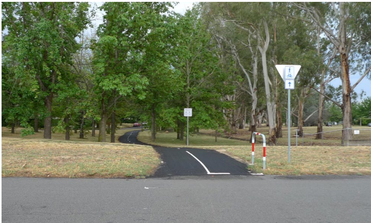
Figure C.1 – Path with minimal termination treatment
