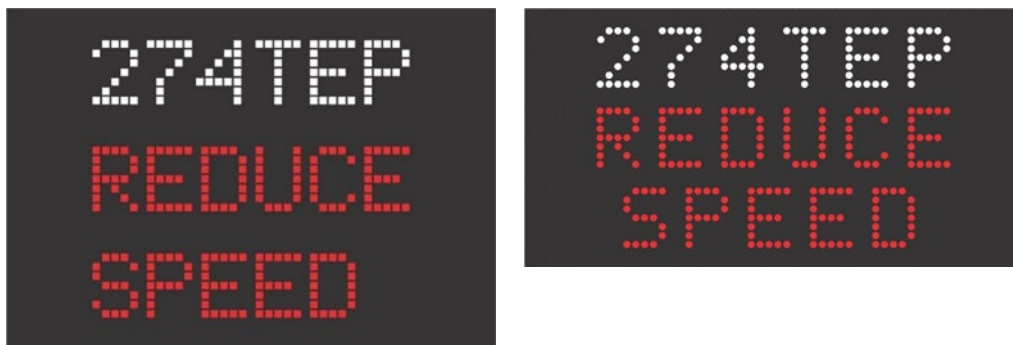
Figure 1.7.4(c) – Variable message sign display examples (more than 10 km/h above the speed limit)
