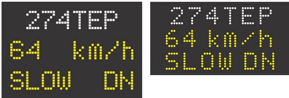
Figure 1.7.4(b) – Variable message sign display examples (up to and including 10 km/h above the speed limit)
