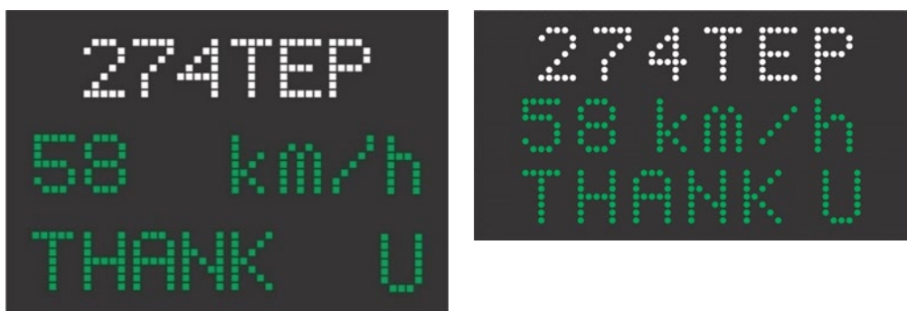
Figure 1.7.4(a) – Variable message sign display examples (equal to or below the speed limit)
