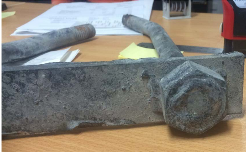
Figure 13-4 – Failed bolt due to fabricated bolt being used instead of forged bolt
