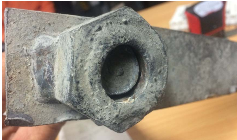
Figure 13-4 – Failed bolt due to fabricated bolt being used instead of forged bolt
