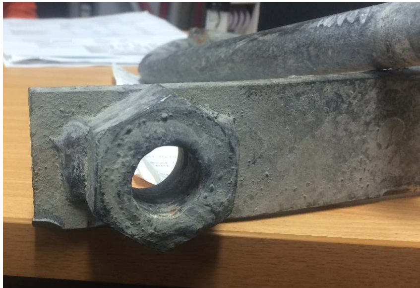
Figure 13-2 – No connection between shaft of bolt and nut in welded bolt
