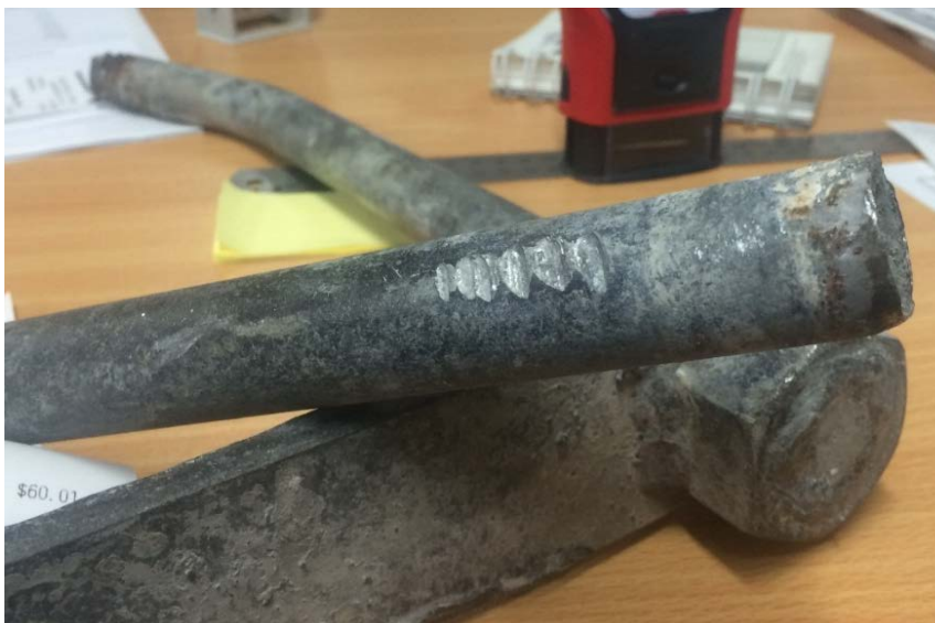
Figure 13-2 – No connection between shaft of bolt and nut in welded bolt
