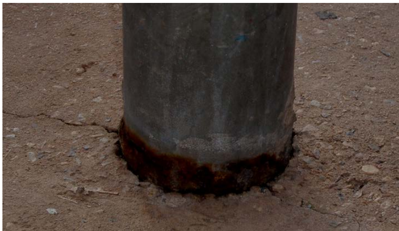
Figure 8.2-2 – Corrosion of buried post
