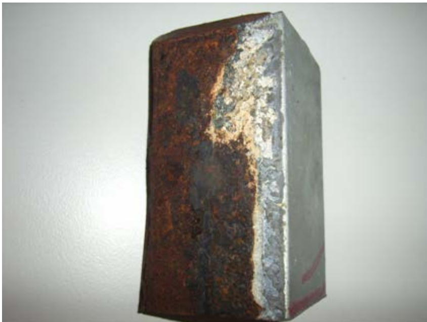
Figure 4 – View of the corrosion when two back to back angles were placed against one another
