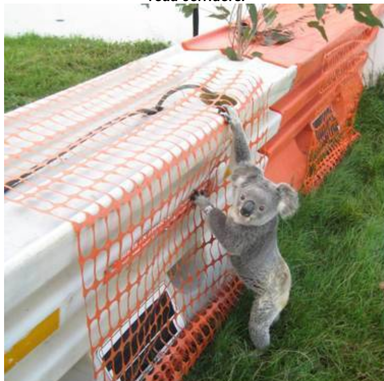
Figure 6.18.11 Koala barrier trial at the Australian Wildlife Hospital, Queensland. Some koalas were able to use parawebbing to climb over the barrier (Scott 2008).
