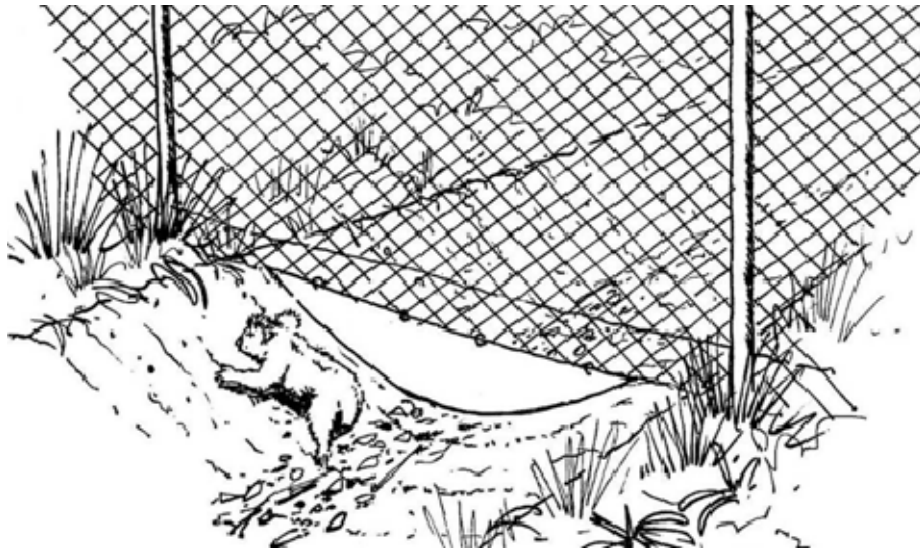
Figure 6.11.3 Flap joined to the bottom of fauna exclusion fencing to prevent fauna penetrating road corridors at drainage line.
